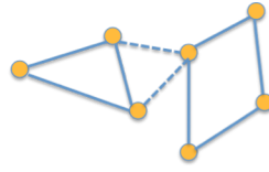
Figure 6: Final touch: replacing edges by short cuts (first possibility). This solution disconnects the graph.
